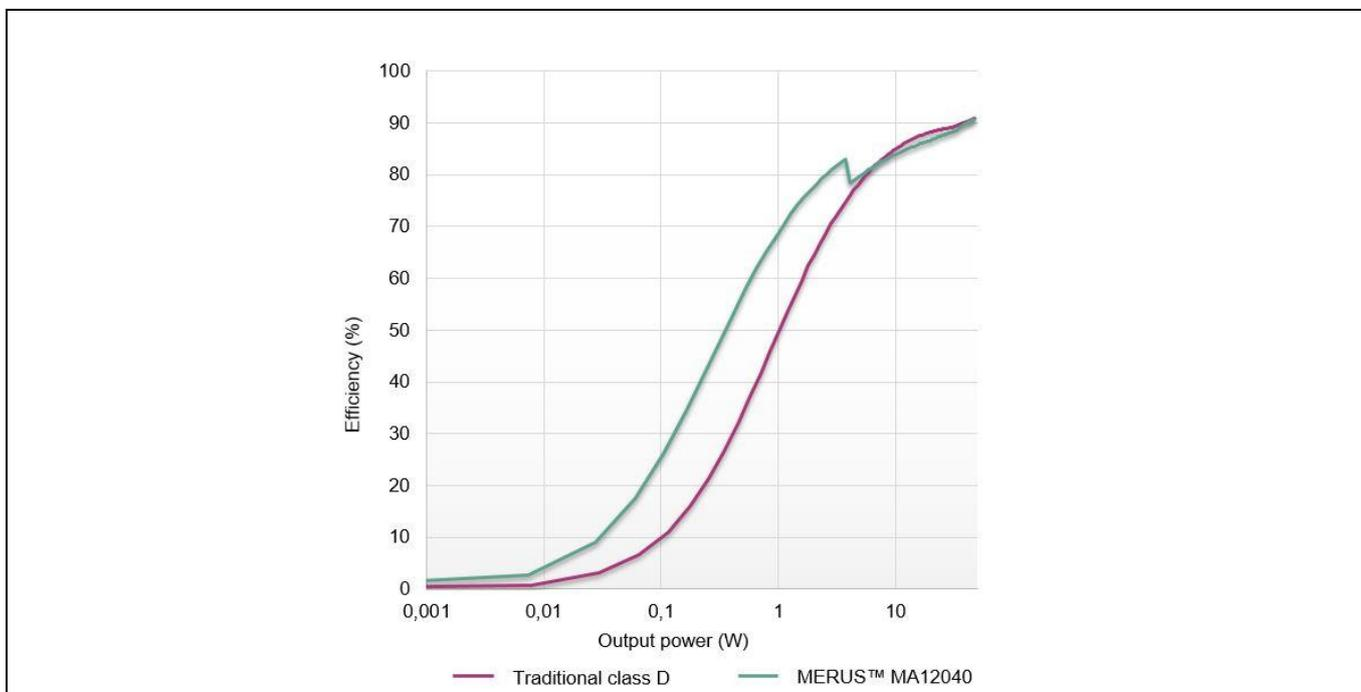
**Figure 10 Efficiency of the MERUS™ MA12040 amplifier**
