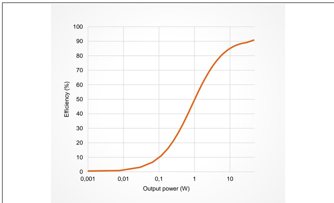
**Figure 2 Efficiency of a traditional class D amplifier**
