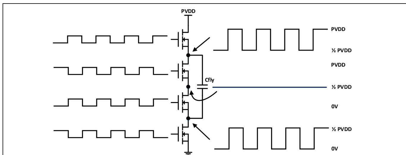
**Figure 8** Multilevel output stage in idle operation
