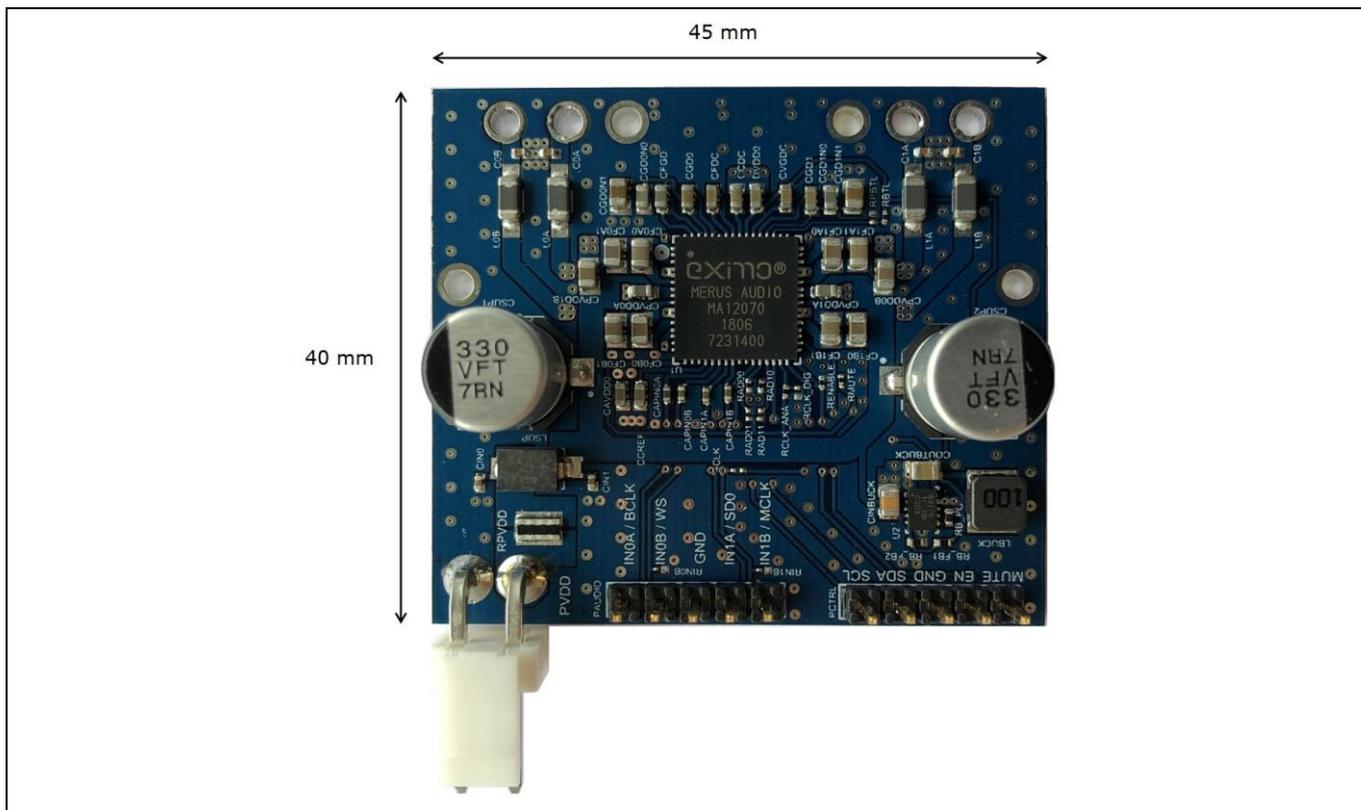
**Figure 12 The Infineon reference design with the MERUS™ MA12040 multilevel amplifier**
