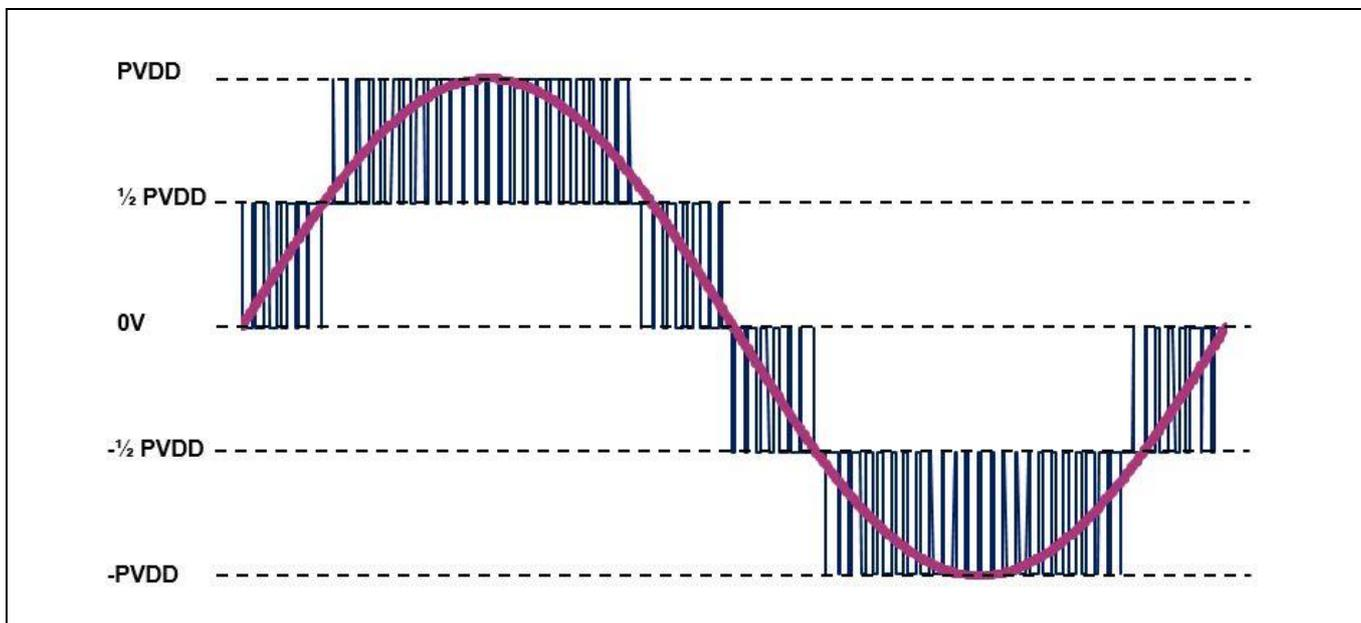
**Figure 6 Full bridge-tied load five-level output signal**
