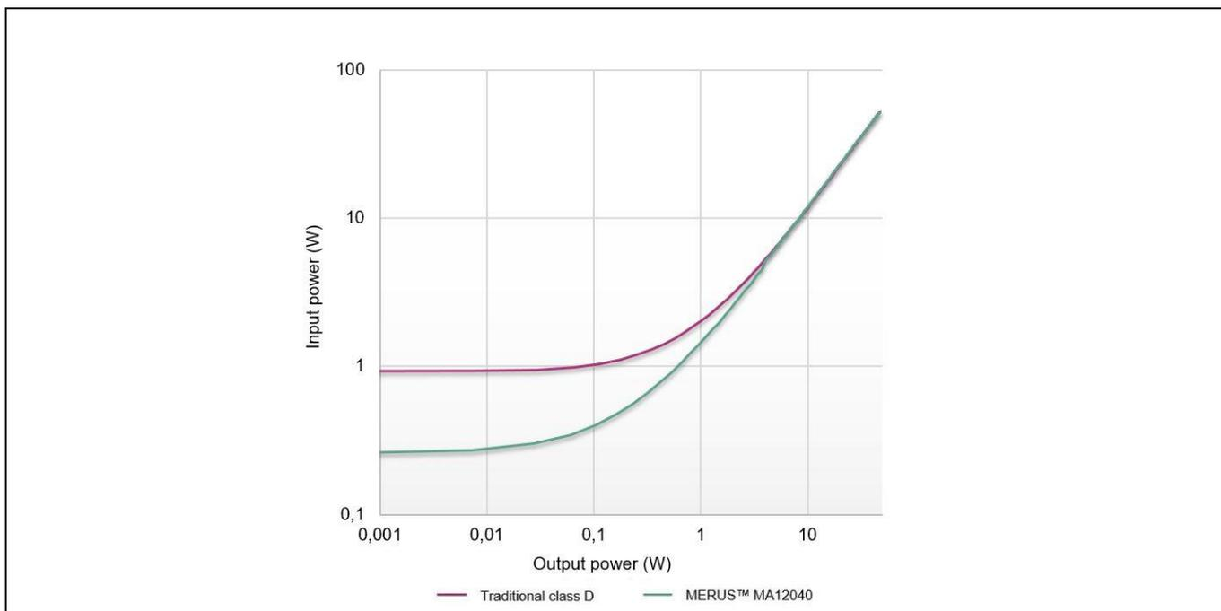
**Figure 9 Power consumption of the MERUS™ MA12040 amplifier**
